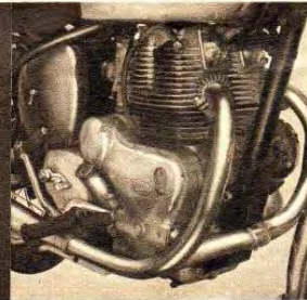
One of Enfields' smoothest twins—the 736 c.c. Interceptor. To fit a rev-meter the small timing-cover plate has to be removed.
